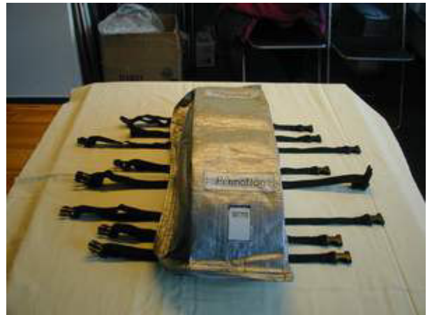
Pic 4: Place the Hygrometer and PermaPack-cylinders in to the PermaBag and close the zip
